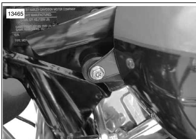
Figure 5. Front Fuel Tank Mounting Tabs Over Braces with Fasteners Installed
