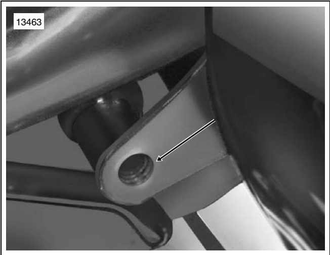
Figure 2. Front Fuel Tank Fasteners Removed
