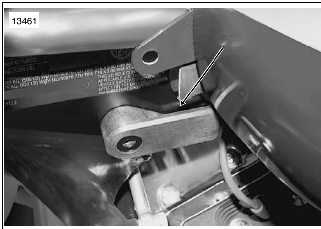
Figure 4. Left Hand Fuel Tank Brace with Cutout
