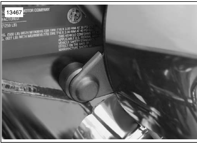
Figure 8. Front Fuel Tank Fastener Boot Installed
